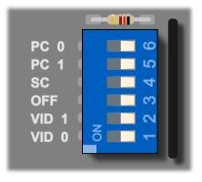
These 2 set the number of inputs the Display Control will cycle through when (data) button is pressed enable/disable automatic screen movement when on/off pressed enable/disable 9hr inactivity shutdown & sleep mode These 2 set the number of inputs the Display Control will cycle through when (video) button is pressed
